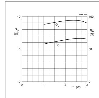
Class-B operation;  $V_{CE} = 24 \text{ V}$ ; f = 900 MHz;  $T_{mb} = 25 \, ^{\circ}C.$
