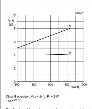
Fig.9 Input impedance (series components) as a function of frequency, typical values.
