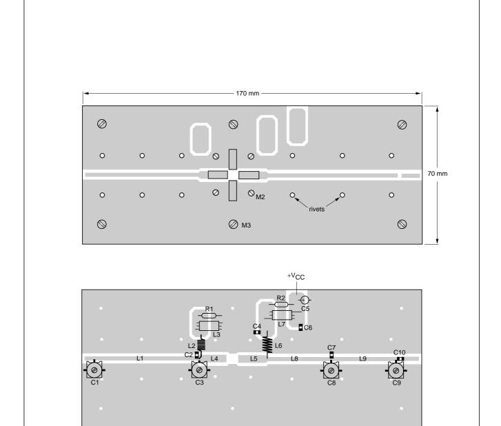
The components are mounted on one side of a copper clad PTFE fibre-glass board; the other side is unetched and serves as a ground plane. Earth connections from the component side to the ground plane are made by fixing screws, hollow rivets and copper straps under the emitters.
