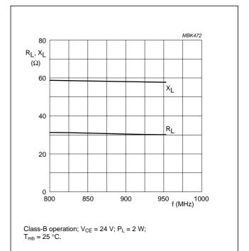
Fig.10 Load impedance (series components) as a function of frequency, typical values.
